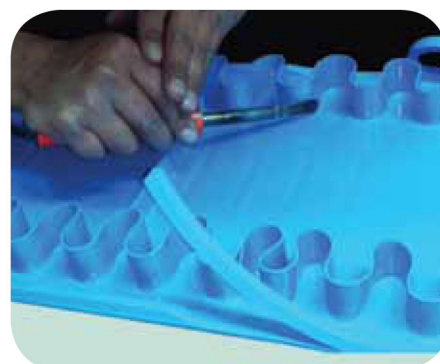
Sidewalls and Guides endless welding
